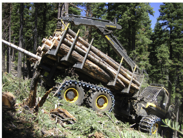
Fig. 3. Cable-assisted loaded forwarder moving uphill on a steep slope within a pilot test at Fremont National Forest, south-central, Oregon, July 2016. Photo Credit: John Sessions.
